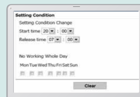
Engine start alarm outside prescribed work time
